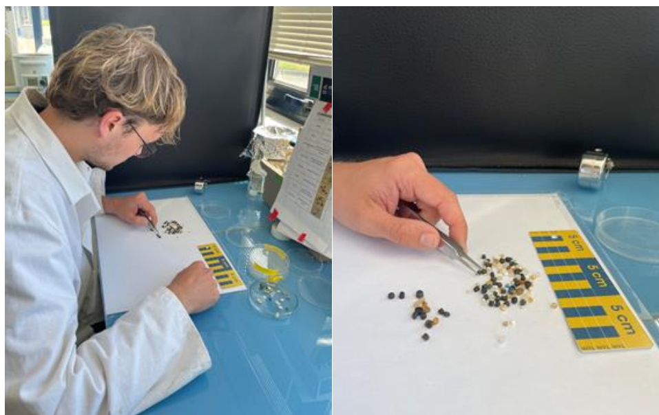
Figure 3 : Manual sorting of a RNS-mP-P sample prior to visual counting ©CEDRE
