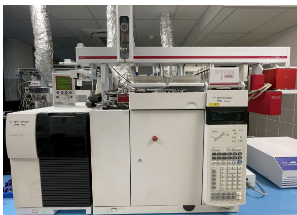
Figure 7: Agilent Technologies 7890A gas chromatograph (Left), thermal Desorption Unit (Gerstel) used in CEDRE laboratory.
