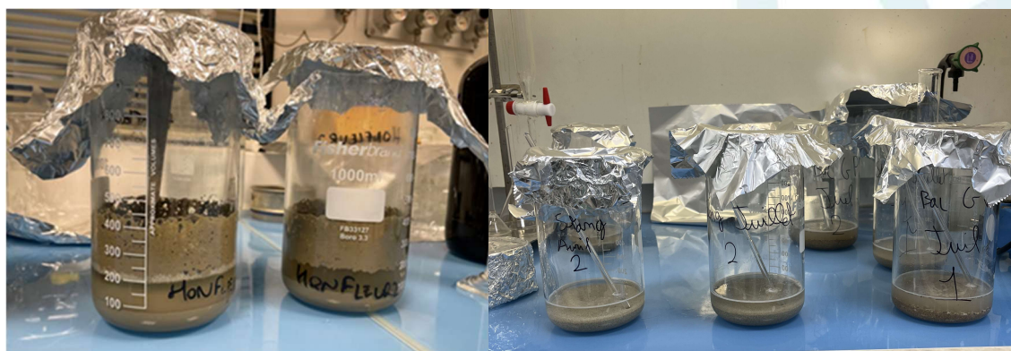
Figure 3 : Digestion of organic matter in sediment samples ©CEDRE. Left: port sediments, right: beach sediments.
